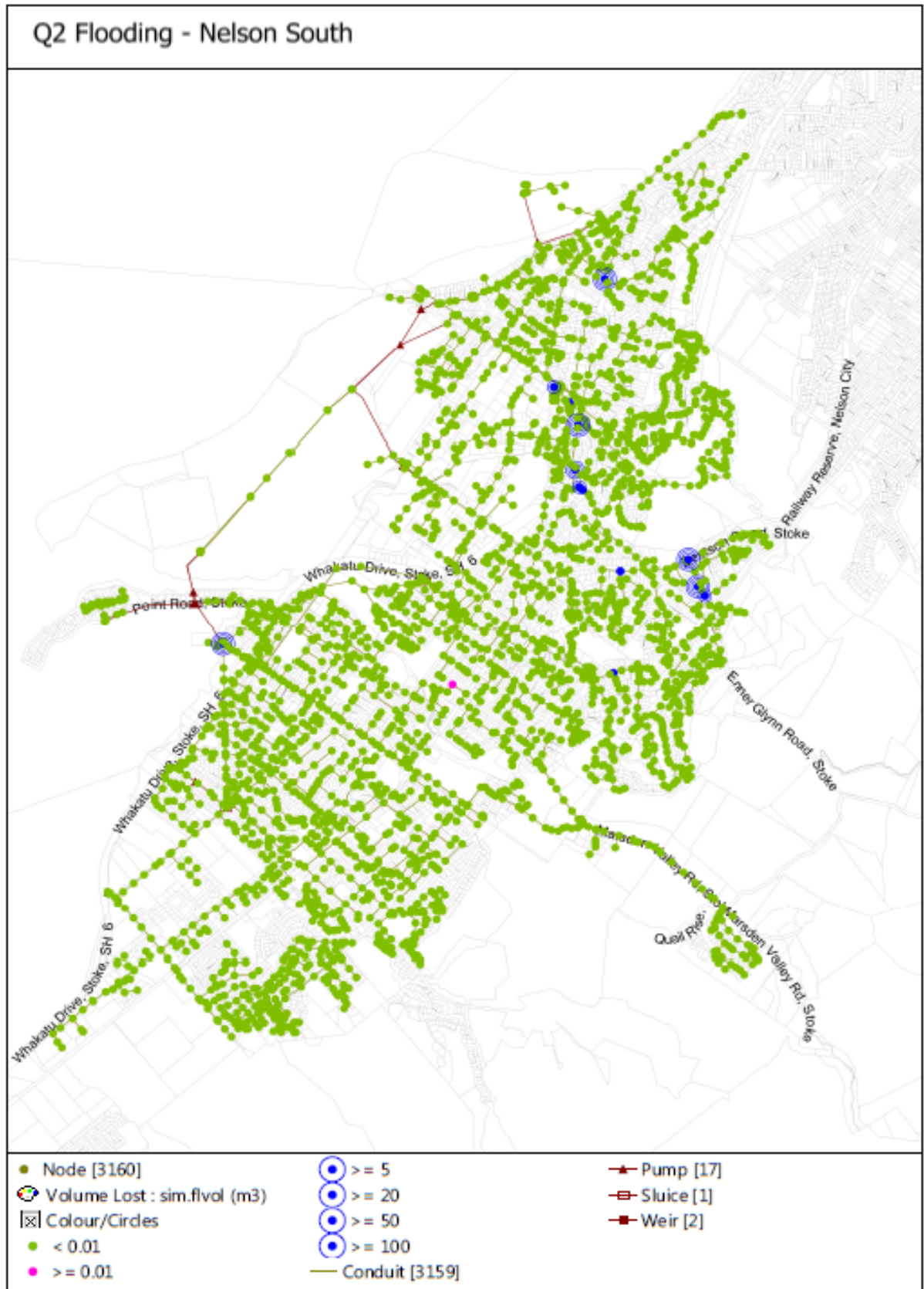
Figure ES-3: Flooding – Nelson South
